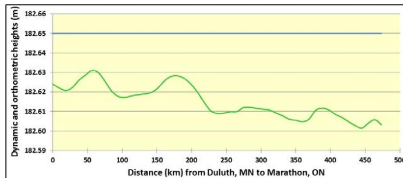
**Figure 3.** Orthometric heights (lower green line) versus dynamic heights (upper blue line) of Lake Superior water surface along a straight line profile from Duluth, Minnesota to Marathon, Ontario, illustrating that orthometric heights are not constant along a level water surface, while dynamic heights are.
