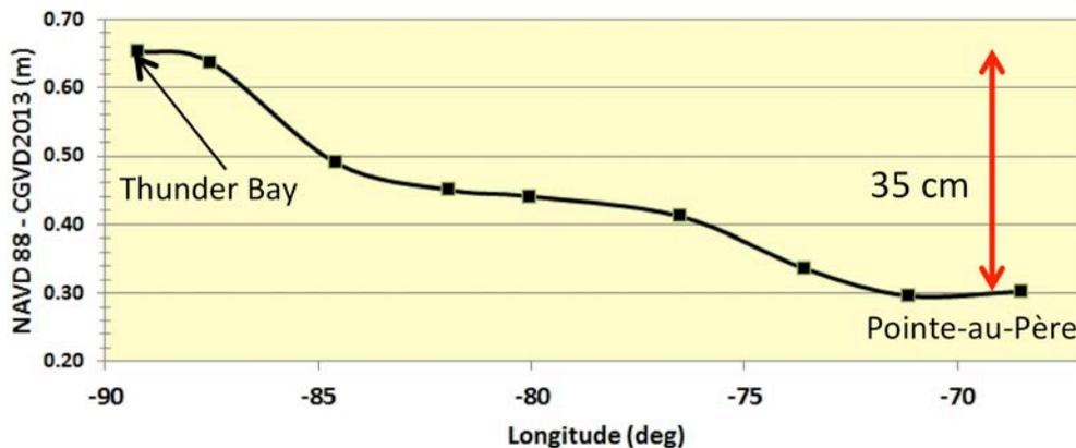
**Figure 1.** Errors in NAVD 88 heights as determined from comparisons with heights in the geoid-based CGVD2013 datum along a leveling profile from Pointe-au-Père, QC to Thunder Bay, ON.
